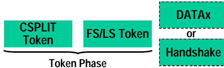
Figure 8-7. Packets in a Complete-split Transaction
